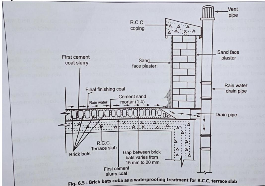
Fig. 6.5 : Brick bats coba as a waterproofing treatment for R.C.C. terrace slab
