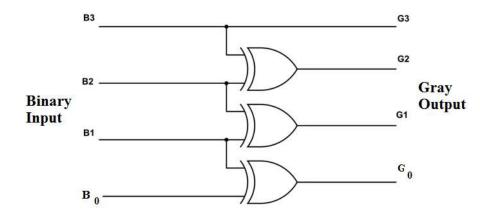
Note: Realization of output equations can be done using Basic or Universal gates
