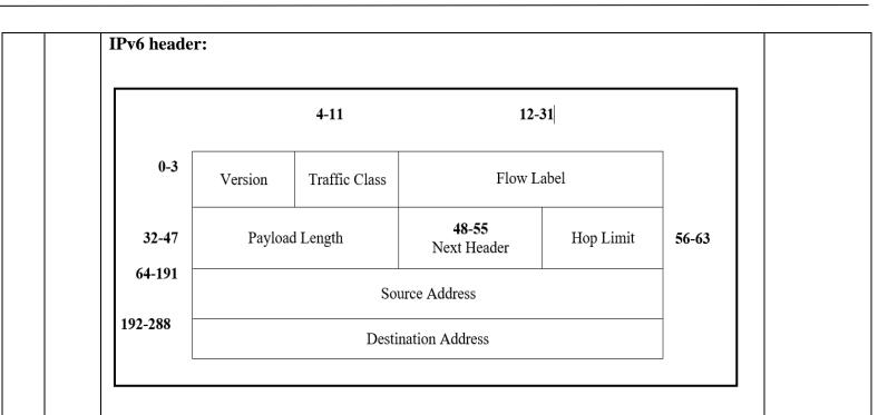
IPv6 fixed header is 40 bytes long and contains the following information.
